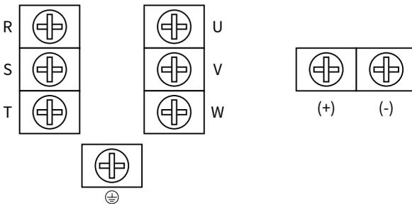
\*Remarks : R/S/T, U/V/W wiring terminals at the bottom of servo drive; (+) / (-) wiring terminals at the top of servo drive
