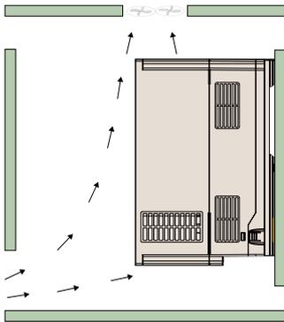
Correct installation position of cooling fan
