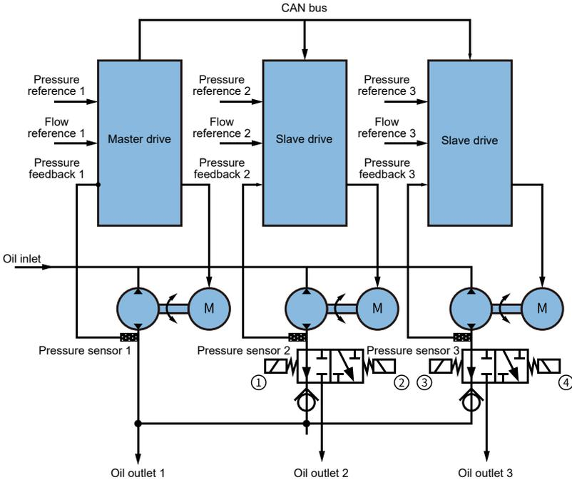
Note: You can ensure the same motor speed through the communication.
