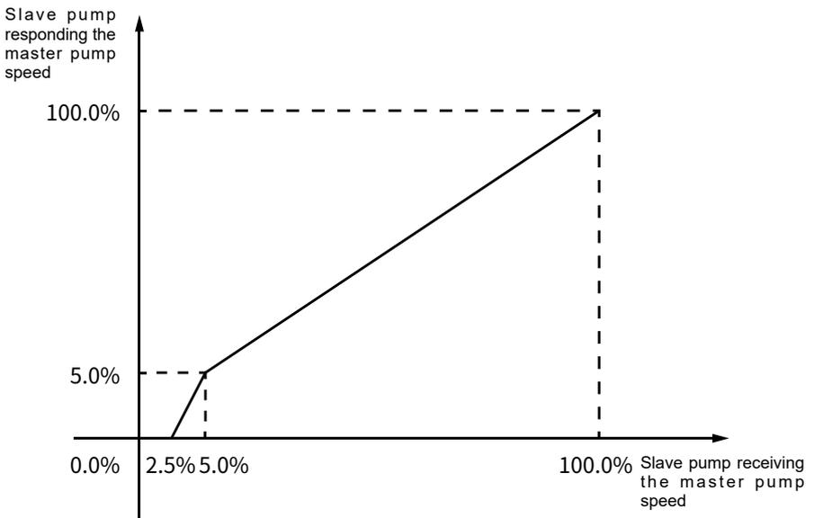
Note : The two multi-pump modes have the same parameter setting for the slave pump response to the master pump speed reference.
