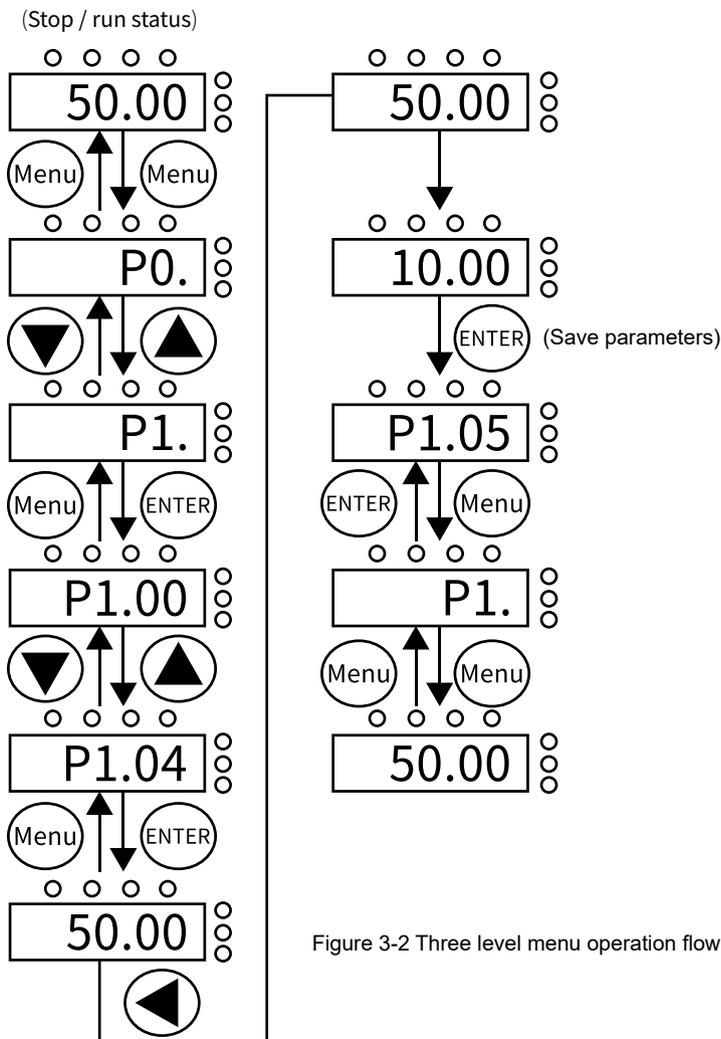
Figure 3-2 Three level menu operation flow chart
