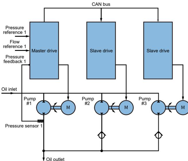
Note: You can ensure the same motor speed through the communication.
