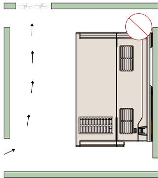
Incorrect installation position of cooling fan
